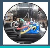
The stage of adjusting the bases of the rotor, delta or star.
